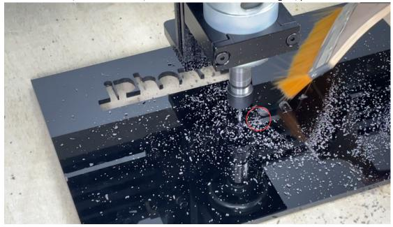
When it finish work, spindle will go back to the original position, so you can turn off spindle or adjust spindle speed down, move the z kit away then take out the cutting result.
