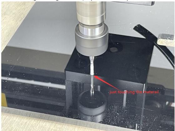
6.On software pls activate Z kit operation button, this button for control Z axis up and down on software, but normally we suggest adjust Z axis by manual with hand wheel.
