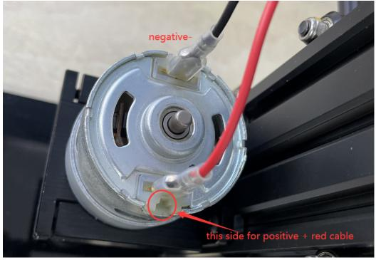
4.Just connect the DC power cable from 24v adapter, we suggest adjust power from 12-19v, donot adjust to 24v for spindle this will easier burnt it.
